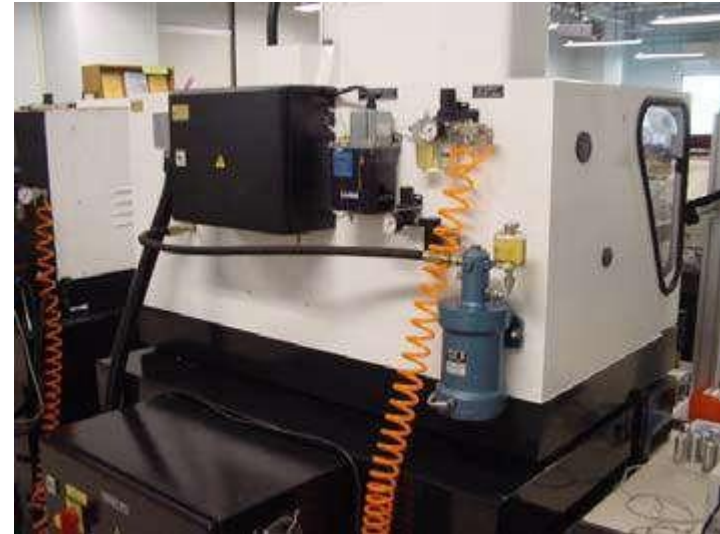
(b) Pneumatic system of an automatic machine
